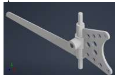
Gambar. 4 Desain steering knuckle
