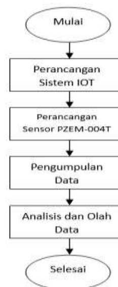
Gambar 1: Diagram Alir Tahapan Penelitian Analisis Sensor PZEM-004T
