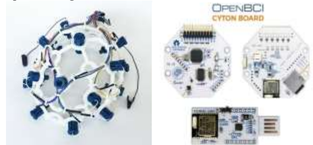
Gambar 3. Helmet EEG Ultracortex Mark IV beserta Cyton Board
